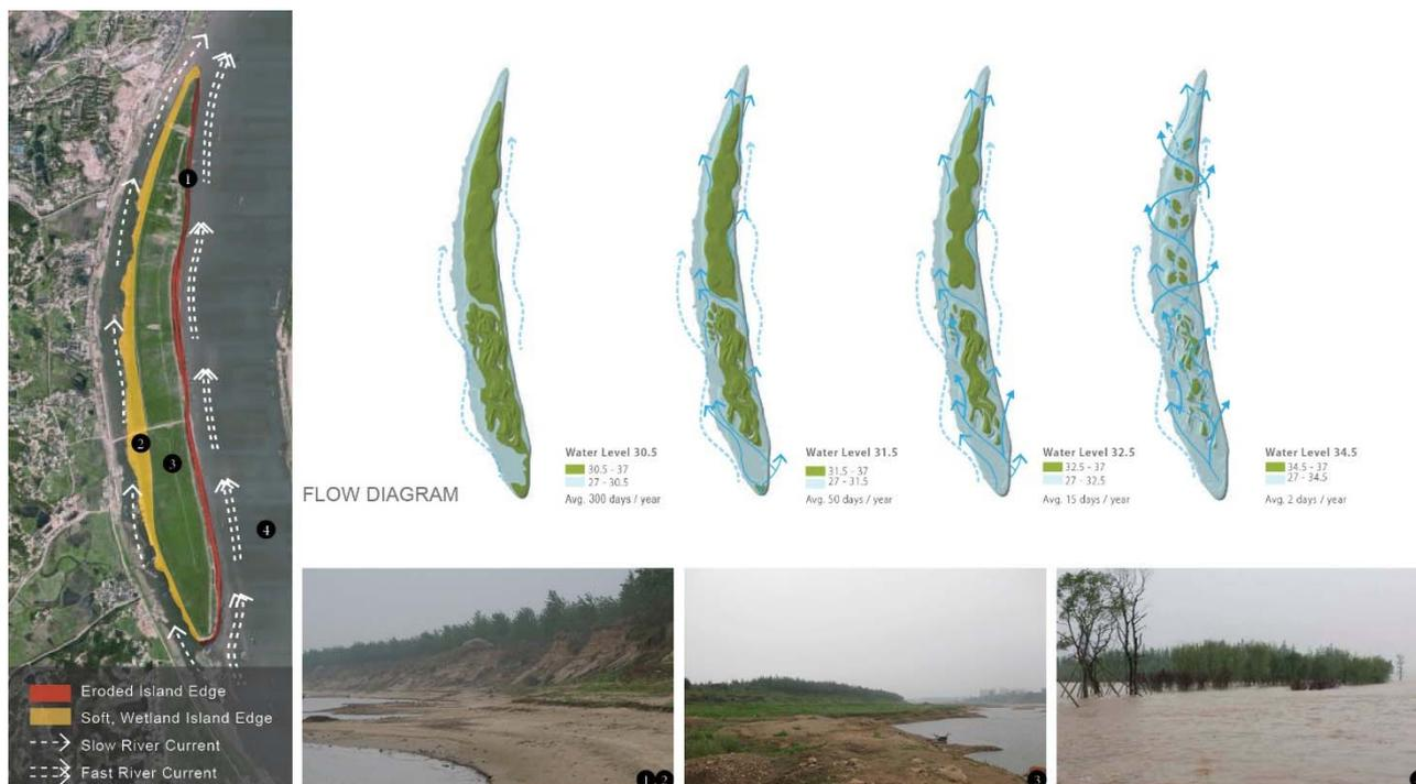
A wider river channel and higher river velocity have led to river bank erosion. Based upon existing topography and 6 meters annual water fluctuations, the design allow rising waters to flow through and over, leaving the river carrying capacity unchanged at flood season.
